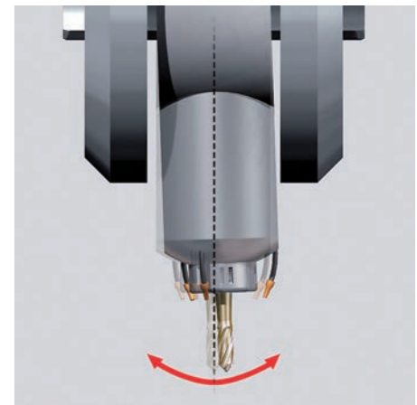
Fault characteristics according to ISO 230-1: EBA
