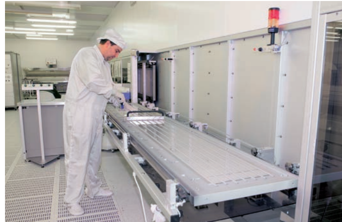
Vacuum machine for application of chromium layers
