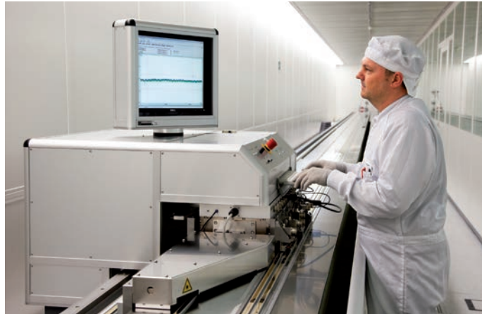
30 m long measuring machine for scale tapes
