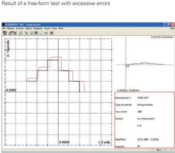
Result of a step response test as an "Xt" graph
