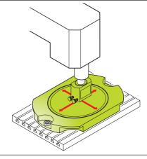
Circular interpolation tests with very small radii and free-form tests provide information on the dynamic behavior of the control, and circular interpolation tests with large radii provide information on the machine geometry.
