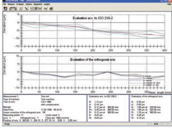
Measurement of the static positioning accuracy as per DIN ISO 230-2 and the guideway error in transverse direction
