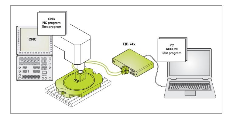
ACCOM automatically detects the beginning of the inspection procedure—for example when a certain distance or angle has been moved from the starting position.
