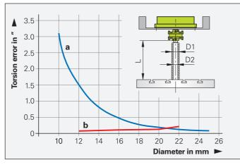
Torsion error of the 100-mm long coupling of an ROD 880 via a a) Solid shaft with various diameters D1
